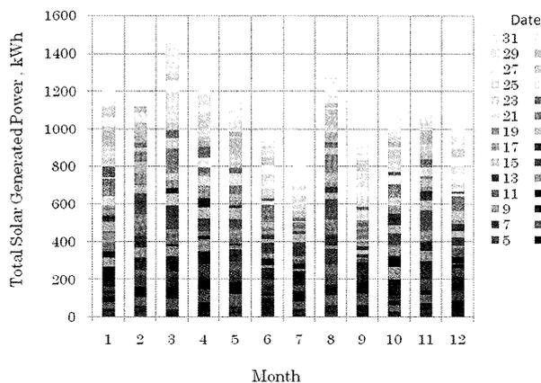
Fig. 1. The total monthly generated solar power.
